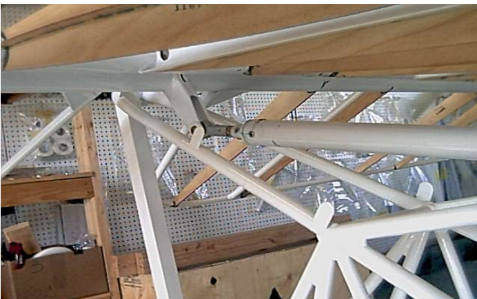
Elevator connection to Push tube
