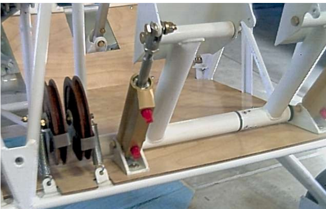
Rudder Pulleys
