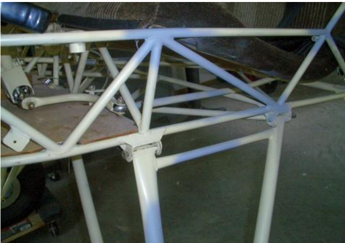
Undercarriage mounting
